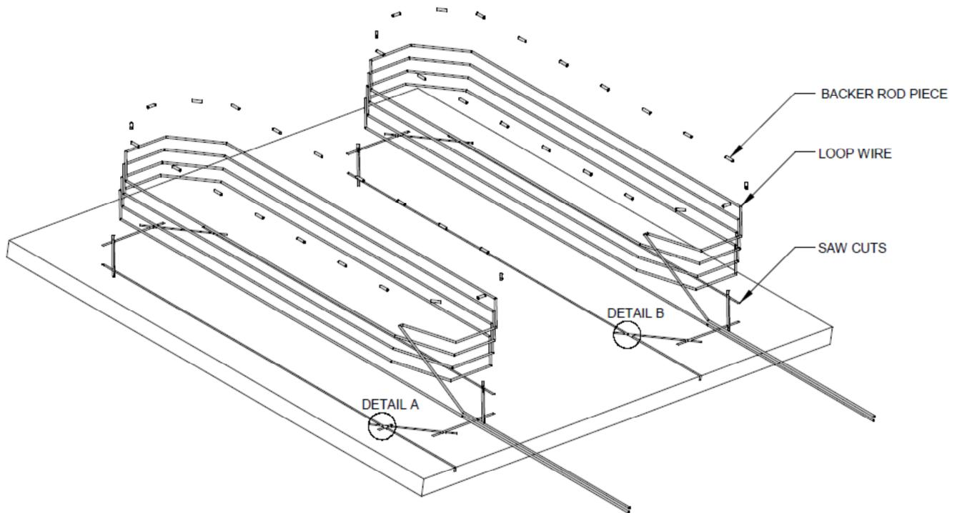
The corners of the loop should be crosscut at a 45° to help prevent damage to the wire insulation during installation and temperature cycling. The angled cuts should be at least 9" back from where the corner would be. The saw cuts should not go any further than necessary to insure that the saw slots are at full depth where they meet.
