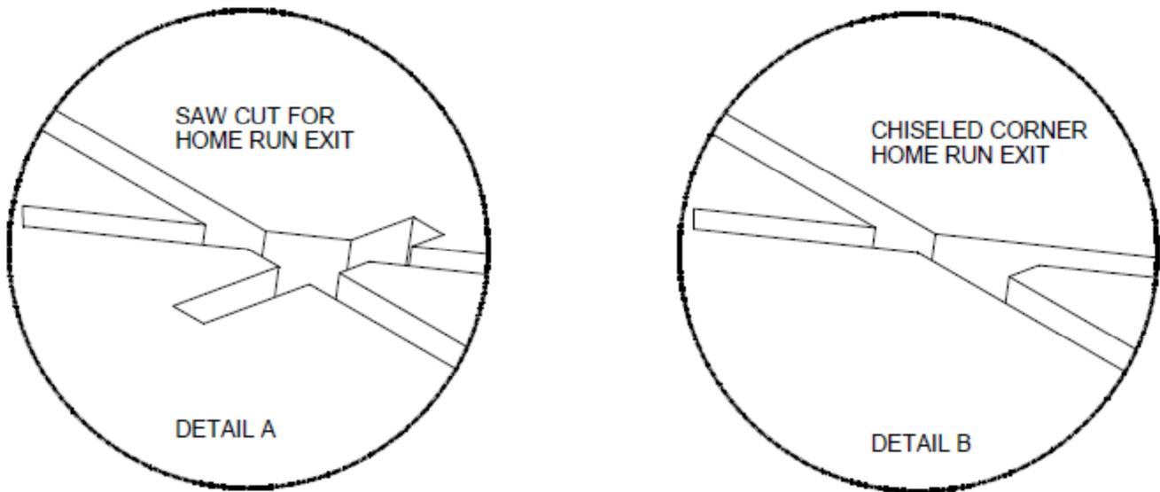
Once the saw slot has been cut, the slot should be cleaned of all loose material. High pressure air should be directed in to the saw slot to remove all debris. This will also help remove dust from the saw cutting operation from the sides of the saw slot. This will allow better adhesion of the loop sealant to the saw slot.
