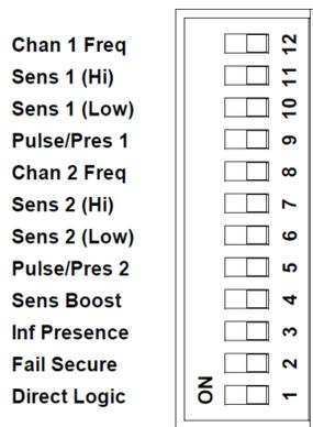
All of the controls for adjusting the configuration of the DSP-20 detector are located on the front panel 12-position DIP switch. There are no internal DIP switches or jumpers to configure.
